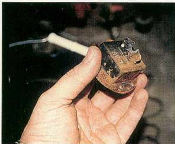
Low water cut-off switch damaged by unidentified leaking water.
