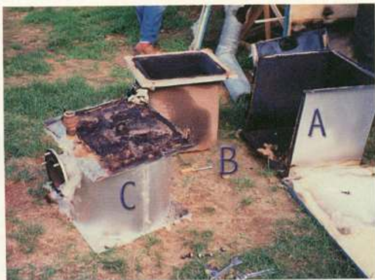
(Above) Dismantled dry base boiler. "B" is the "tub-like" refractory in this type of boiler.
